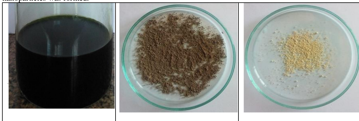
Fig. 1. a) Ethanolic leaf extract of Nyctanthes arbor tritis , b) chemically synthesized TiO 2 after calcination c) green synthesized TiO 2 nanoparticles after calcination.
